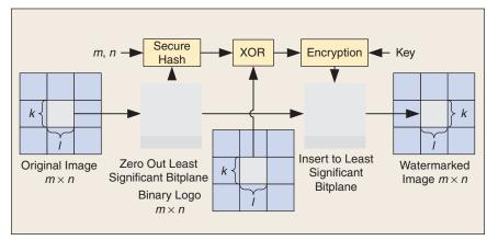
▲ 5. Block-based fragile watermarking scheme for image authentication [10].
