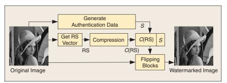
▲ 6. RS lossless watermarking for authentication [15].
