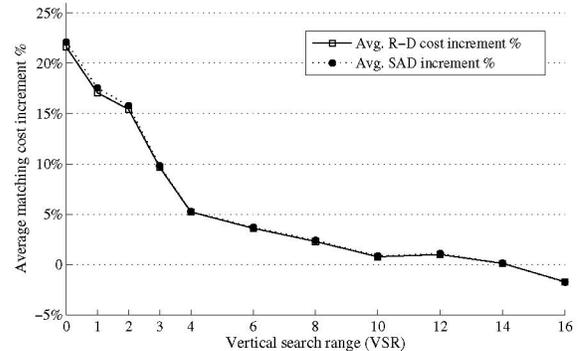
Fig. 5. Average matching cost increment % versus VSR.
