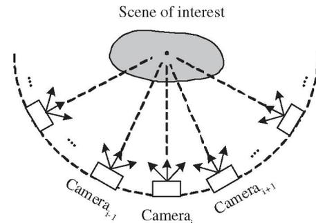
Fig. 1. A convergent multi-view camera setup.
