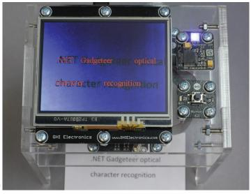
Figure 7. Optical character recognition (OCR) device. (a) The OCR device has a camera facing down toward the surface it is resting on. (b) The display on the OCR device shows an image of some printed text with the OCR'd characters correctly overlaid in red. This is implemented using the Project Hawaii cloud-based OCR service.
