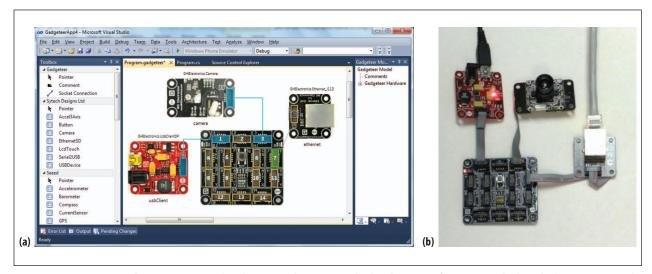
**Figure 2.** An Internet webcam constructed with .NET Gadgeteer. (a) The hardware configuration, which includes an RJ45 module for a wired Ethernet connection, is entered graphically in Visual Studio. When a module connector is selected, compatible mainboard sockets are highlighted in green to aid the user in wiring up the design. (b) The corresponding physical hardware of the completed webcam.
