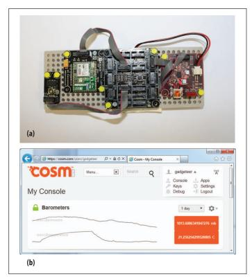
**Figure 6.** Prototype device created with Gadgeteer. (a) The device periodically stores temperature and pressure readings using the cosm Web service via Wi-Fi. Note that the prototype is assembled using a perforated plastic baseboard; yellow plastic pop-rivets attach the Gadgeteer modules to the baseboard. (b) Data plots collected over a 24-hour period.
