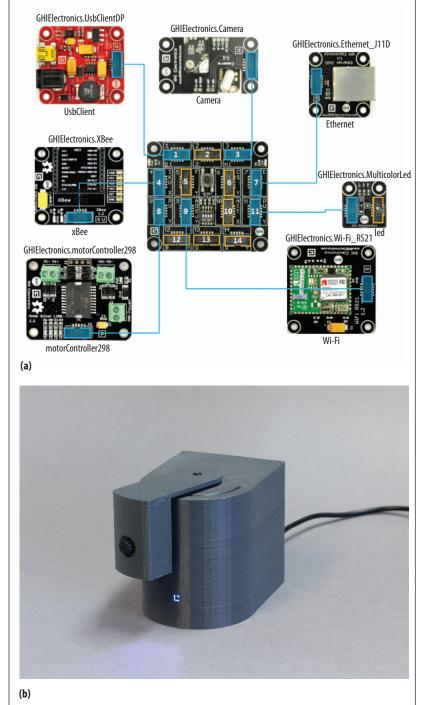
**Figure 4.** Web-controlled camera. (a) The remote-controllable networked camera with servo-controller pan mechanism. (b) A 3D-printed plastic enclosure houses the electronic modules.
