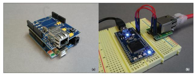
Figure 1. Connected-device prototyping tools: (a) Arduino device prototyping platform with Ethernet shield and (b) the mbed embedded development platform.
