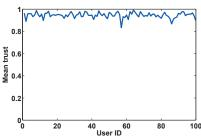
Fig. 3. Under benign settings the packet losses due to wireless effects affect the mean trust of all UEs to the same degree.
