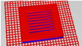
**figure 2.** masking test structure (ABS: blue, PLA: red)
