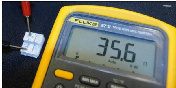
**figure 3.** a printed 3D dimensional trace
