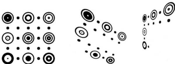
Figure 3. The pattern with independent features and dependent features. The left is the original pattern. All features in this pattern are numbered 0 to 24, from left to right, top to bottom. The center is the pattern after a perspective transform. The right is the pattern after another transform. The features 0, 2 and 4 are visible independent features. The features 1 and 3 can be found using the cross ratio.
