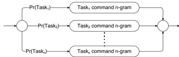
Figure 8: HMM/CFG model’s call-routing topology.
