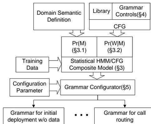
Figure 1: SGStudio architecture. At the center is the HMM/CFG composite model that incorporates domain knowledge, in the form of domain semantic definition and PCFG rules for domain-related concepts. The model can be configured with the configuration parameters to produce different grammars according to different application scenarios.
