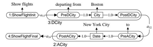
Figure 4: A zoomed-in view of a state alignment for the phrase “departing from Boston to New York City” according to the network topology in Figure 3. The output distribution of the rectangle states follows a PCFG, and that for the rounded rectangle states follows an n-gram model.
