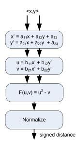
**Figure 2:** Four stage signed distance function for second order *Bezier curve.*
