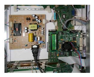
**Figure 4:** Rear view of physical apparatus including one of the six LCD panels with power supply (left) and FPGA development kit (lower right) attached.
