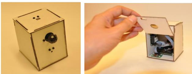
**Figure 5.** Cardboard is used to prototype a new type of passive infra-red sensing device [11]. Nylon screws hold the Gadgeteer components in place (at right).
