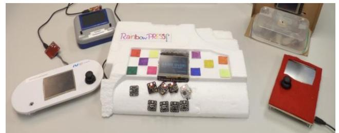
**Figure 3.** Prototype devices produced during a school pilot use a wide variety of materials to produce the required form-factors. These include (from left-to-right) printed cardboard, vacuum-formed plastic, expanded polystyrene, cardboard/plastic, and felt-over-cardboard.
