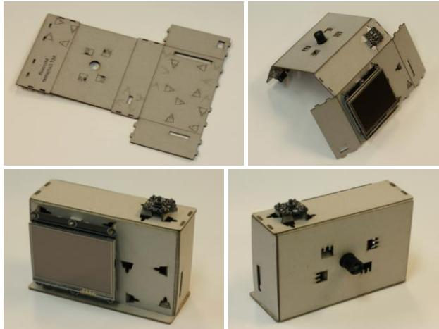
**Figure 6.** A cardboard digital camera case. Modules are mounted directly onto fold-out pillars and the unit fastens together in a ‘tongue-and-groove’ style; the display and pushbutton are external and everything else is internal.
