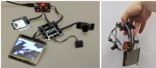
**Figure 1.** Functional prototype of a digital camera.
