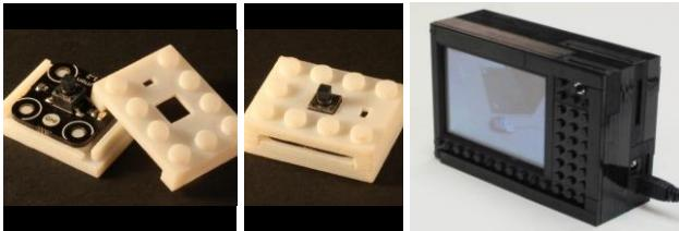
**Figure 4.** Enclosing a Gadgeteer module in a ‘wrapper’ makes it compatible with off-the-shelf construction systems. It is then possible to build prototypes such as this digital camera (shown at right) relatively quickly.
