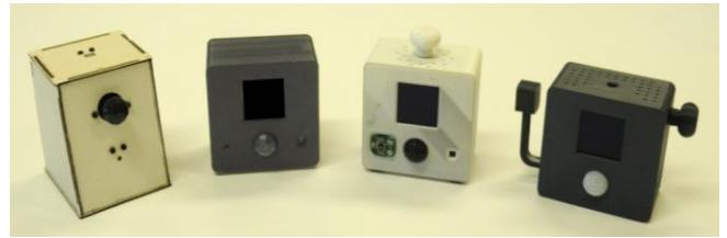
**Figure 10.** Iteration from cardboard to 3D printer.
