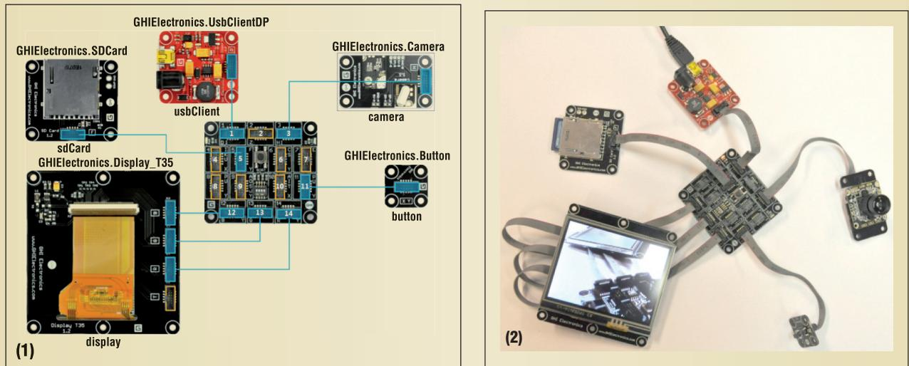
Figure A. Creating a digital camera using .NET Gadgeteer: (1) the graphical configuration tool and (2) the corresponding hardware.
