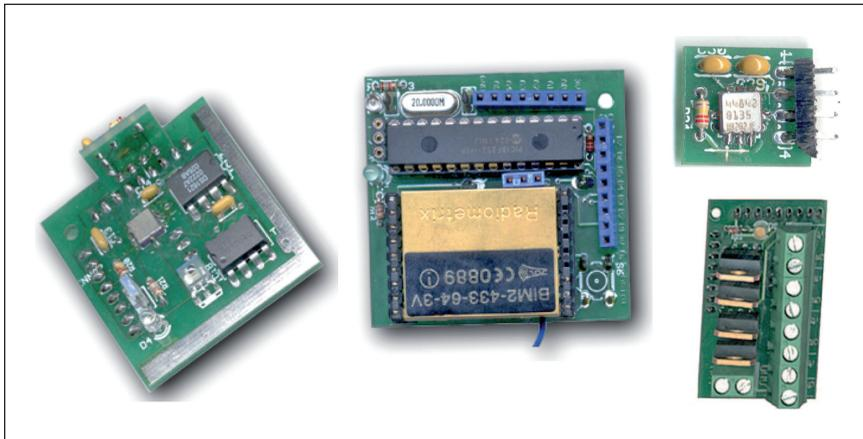
Figure 1. Smart-Its—an early prototyping platform developed in 2001.
