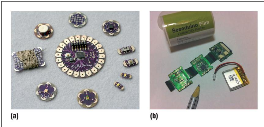
Figure 2. Arduino has revolutionized electronics development, and a very active community has evolved the hardware platform from the original standard printed circuit board (PCB) form-factor to include (a) wearable devices, such as Lilypad (photo courtesy of Leah Buechley) and (b) very small, flexible devices, such as Seeeduino film.
