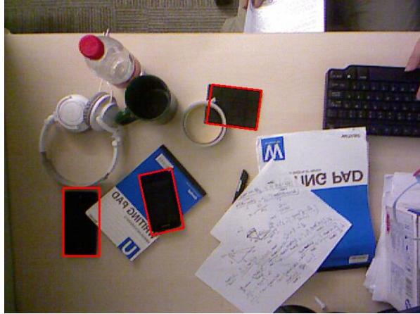
Figure 7: An example to illustrate that AutoCharge is able to correctly identify rectangle objects in a picture together with many other objects.
