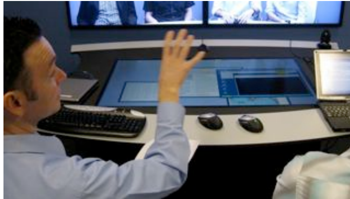
Fig. 5. Table rim in BISi designed to accommodate keyboards, pointing devices as well as laptops that people might need to bring into the collaboration without interfering with the horizontal touch surface.
