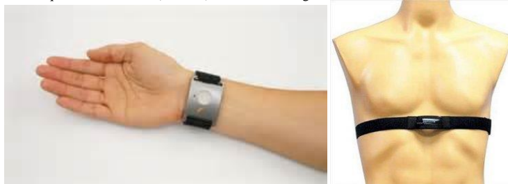
Fig. 1. Affectiva Q Sensor (left) and Zephyr HXM ElectroCardioGram monitor (right)
