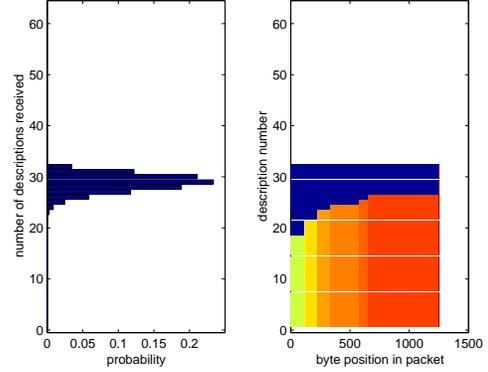
**Fig. 3.** Binomial(32, 0.10) distribution and matched PET packetization. The light-colored bands correspond to source bytes and the dark ones to FEC.
