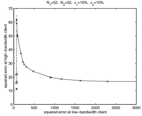
**Fig. 9.** Expected distortion of low-bandwidth client vs. expected distortion of high-bandwidth client for different layered MDC schemes, with 10% packet loss.  $N_1 = N_2 = 32$ .
