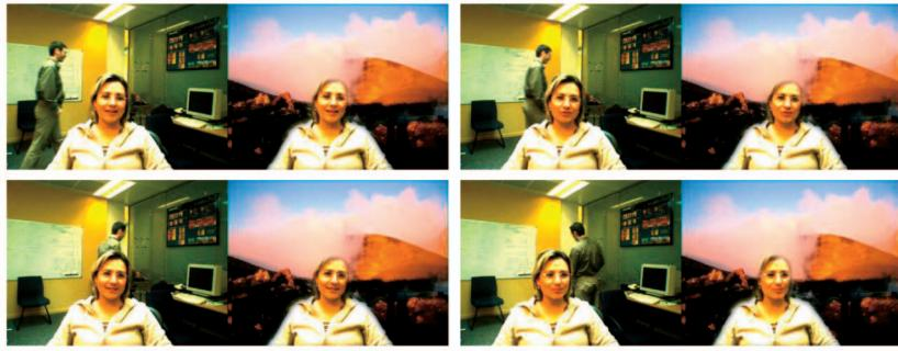
Fig. 12. Background substitution on the “IU” test sequence from [13]. Original and corresponding segmented frames with background substitution. People moving behind the person in the foreground are correctly classified as being in the background.
