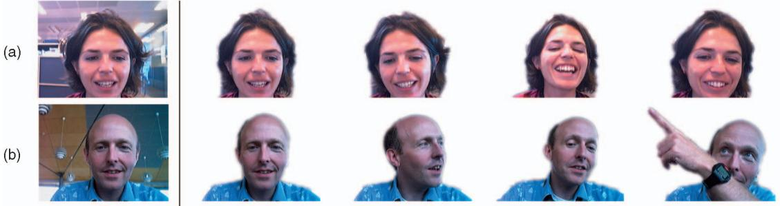
Fig. 10. Segmentation results. (a) An original frame and four segmented frames for test sequence “41.” (b) An original frame and four segmented frames for test sequence “54.” Border matting [25] could be applied here to improve the hair regions. This paper is concerned with binary segmentation only.
