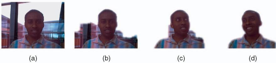
Fig. 14. Self-initialization. (a) Original frame from test sequences “58.” Because of harsh lighting conditions, the segmentation problem is challenging. (b)-(d) Segmentation for different frames in chronological order. After an initial “burn-in” period, the algorithm converges to the correct Fg/Bg separation. A “clean” background image or other types of initialization was not necessary.
