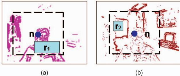
Fig. 6. Shape filters applied to motion bands. (a) and (b) Two motion bands with rectangular masks  $r_1$  and  $r_2$  (centered at the same pixel  $n$ ) superimposed. Given  $n$  and the shape filter  $(k, r)$ ,  $v_n(k, r)$  counts the number of pixels associated with the texton  $k$  within rectangle  $r$  (see text).
