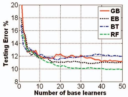
Fig. 8. Comparing accuracy of classifiers. Testing unary accuracy with respect to the complexity of the ensembles in one trial. Five trials have been taken and RF has consistently outperformed the GB, EB, and BT algorithms.
