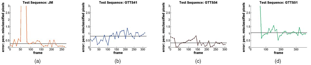
Fig. 13. Accuracy of segmentation. (a) The percentage of misclassified pixels on the “JM” test sequence from [13]. Note how the system promptly recovers from possible mistakes. The median error (horizontal line) is well below 0.5 percent. (b)-(d) The percentage of misclassified pixels for test sequences “41,” “54,” and “51,” respectively. (d) After an initial “burn-in” period, the segmentation converges to a good accuracy level (around or below 1 percent of misclassified pixels).
