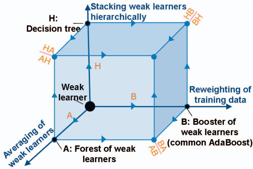
Fig. 7. The tree-cube taxonomy of classifiers captures many classification algorithms in a single structure (see text, for details).
