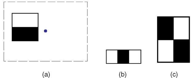
Fig. 5. Some shape filters used in [33], [39], and/or [27]. (a) A shape filter composed of two rectangles (shown in a detection window centered at a particular pixel). (b) and (c) Shape filters composed of more rectangles.
