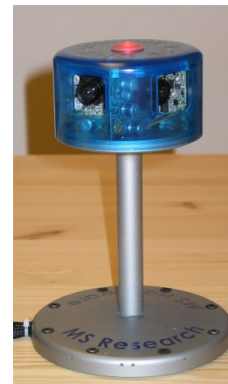
Figure 5: RingCam: an inexpensive omnidirectional camera and microphone array designed for capturing meetings.
