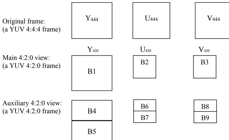
**Figure 2.** Top: Representation of an original frame in YUV 4:4:4 format. Bottom: Decomposition of the frame into two YUV 4:2:0 views.
