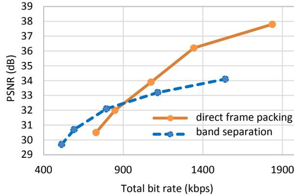
**Figure 3.** Rate-distortion performance comparison between the direct frame packing and band-separation approaches for a fixed main frame bit rate using a Microsoft AVC encoder with a screen content sequence of resolution  $1920 \times 1200$  and length 57 frames, at 30 fps. Auxiliary frame QP varies from  $-12$  to  $+4$  relative to main frame QP, which in this case is set to 39. The bit rate for the main view is 445 kbps, with a PSNR of 31.3 dB.
