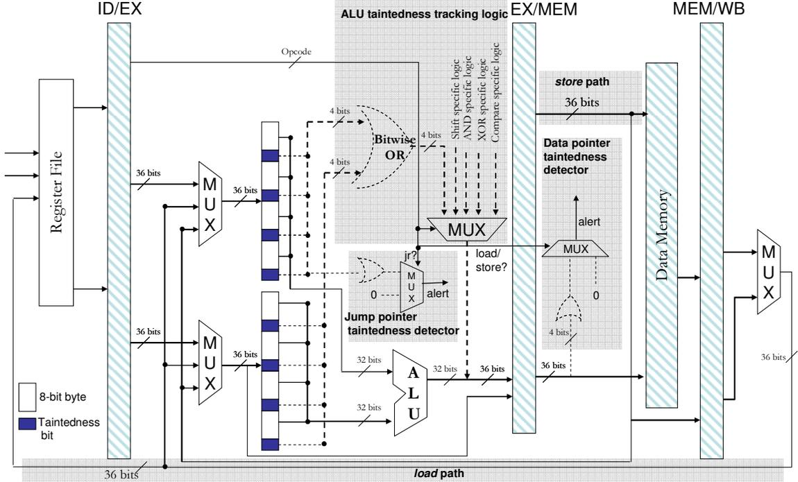
Figure 3: Architecture Design of Pointer Taintedness Tracking and Detection
