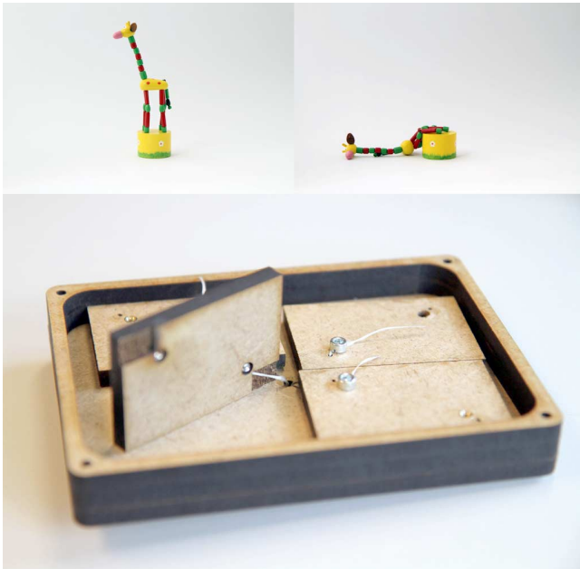
Figure 1. Inspiration and Slacker device. The internal parts can be “clutched” (loose or solid).
