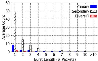
Figure 9: Distribution of packet loss burst length.
