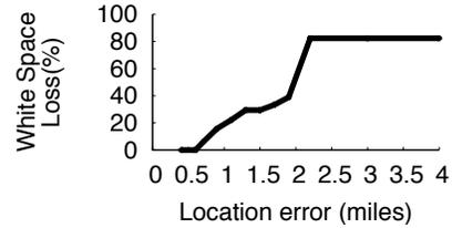
Fig. 4. The impact of location errors on the loss of white spaces.
