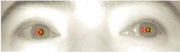
Figure 4: An example of detected glints and pupil center.
