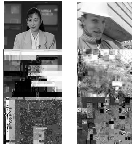
Figure 1. Encryption visual effect. Top: the original. Middle: selective encryption. Bottom: full encryption.
