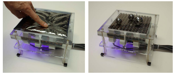
Figure 1. FerroSynth platform showing, (i) interaction with a ferrofluid bladder, and (ii) large ball bearing interface.
