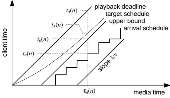
Fig. 1. Coding Rate Control Model
