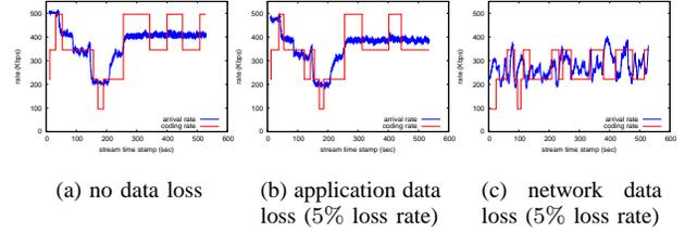
Fig. 4. Performance Impact of Data Loss (over TFRC protocol)
