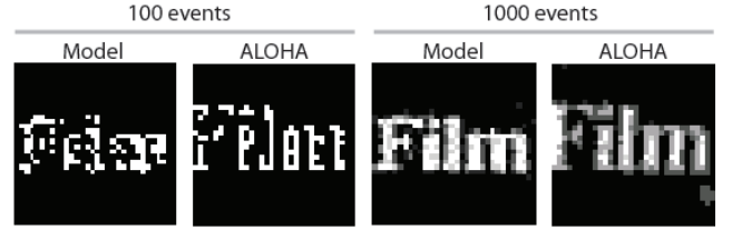
Figure 4: Comparison between the output of the AER model and that of the ALOHA imager.
