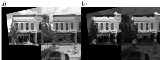
Figure 9. a) Query Image Warped onto Search Image Using Homography; b) Correlation Mask around Matching Feature Points. Correlation Coefficient for Example = 0.8609
