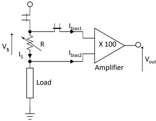
**Figure 6: Setup for measuring sleep currents**
