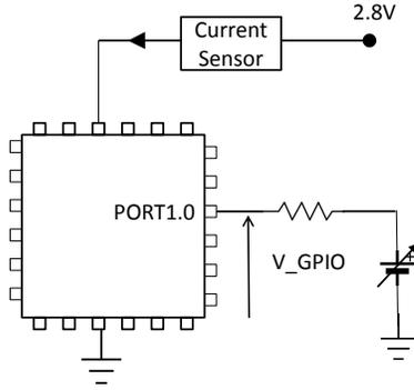
**Figure 7: Setup to measure the impact of GPIO voltage on the processor sleep current.** The MSP430F5438 GPIO pin PORT1.0 was configured as an input, and a variable voltage was applied to it. All the other GPIO pins were configured as outputs.
