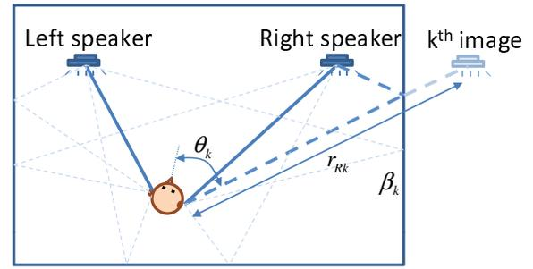
Fig. 3. Acoustic paths between two loudspeakers and the listener’s ears with reflections.
