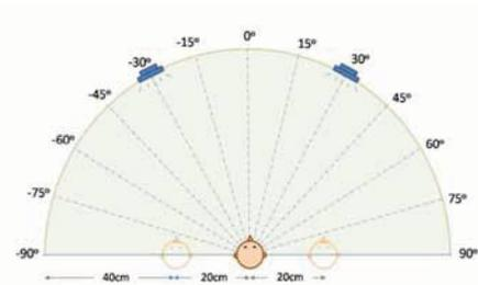
Fig. 5. The listening test configuration.
