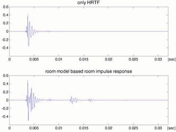
Fig. 4. Room impulse response computed with HRTF only and with the proposed scheme based on room modeling.
