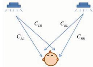
Fig. 2. Acoustic path between two loudspeakers and the listener’s ears.
