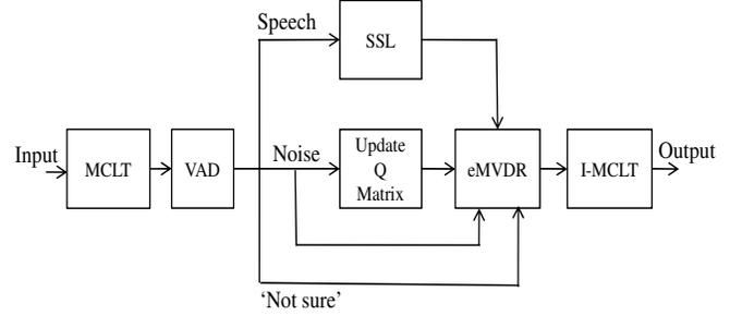
Fig. 3. Block diagram of the eMVDR beamforming
