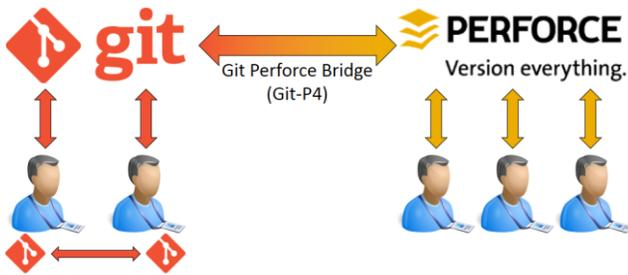
**Figure 2: The architectural diagram for Git-P4.** The developers on the left use Git. They synchronize with either the main Git repository (Git logo at the top left) or their peer’s private Git repositories (small Git logos at the bottom left). The developers on the right use Perforce and only interact with the main Perforce repository. Git-P4 synchronizes the main Git and Perforce repositories in both directions.
