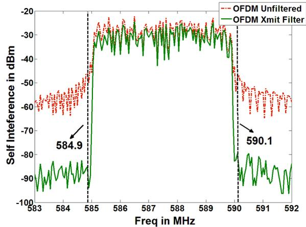
6: Spectrum of transmission with and without filters
