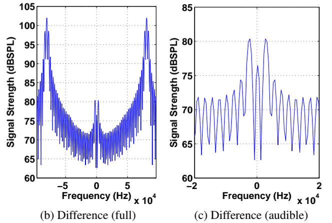
**Fig. 2.** Simulation results of a 39KHz and 41KHz colimated beams. (a) Spectrum of linear and nonlinear simulation from FDTD method. Note how similar the two are; (b) Spectrum of difference signal between the linear and nonlinear simulations in full frequency band. Note the audible signal (around 2KHz) is now above the noise floor; (c) Spectrum of difference signal between linear and nonlinear simulations zoomed in for audible frequency band.
