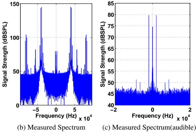
**Fig. 3.** Measurement results: (a) measurement setup for an 8 by 8 parametric speaker array in anechoic chamber using a 1/4 in B & K reference microphone; (b) measured spectrum of this parametric speaker array; (c) measured spectrum zoomed in for audible frequency band.
