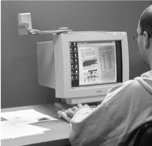
Figure 3: The CamWorks system in use. A digital video camera captures images of a document on the desk, from which the user can select text and image segments for copying into an electronic document.
