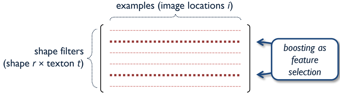
Figure 3.14: Boosting as feature selection. The Joint Boost algorithm acts on a matrix of shape filter responses v_{[r,t]}(i) , and iteratively picks out a feature dimension corresponding to a particular shape filter. The algorithm also selects a set of classes \mathcal{C} between which the chosen shape filter is shared. In this illustration, after two rounds, two shape filters have been selected from the pool of six. For the datasets considered in this work, thousands of shape filters are selected from a pool of hundreds of thousands.
