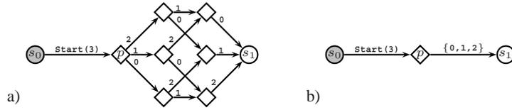
**Fig. 2.** a) Test subgraph obtained by exploring the extended chat model with 3 clients up to the posting phase; transitions from passive states (diamonds) are labeled by the respective client entering the session. b) Same subgraph after compression.
