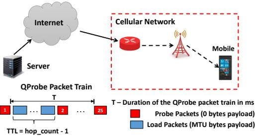
Figure 2: QProbe packet train with tiny probe packets and large load packets. TTL for load packets expires 1-hop before cellular network and get dropped en route.
