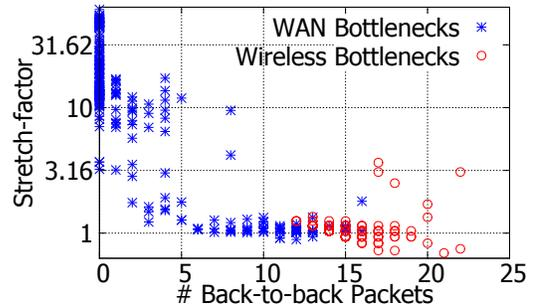
Figure 5: # Back-to-back packets and *stretch-factor* for 489 *QProbe* runs. (Y-axis is in log scale.) WAN bottlenecks result in low # back-to-back packets and high *stretch-factor* while wireless bottlenecks show the opposite behavior.
