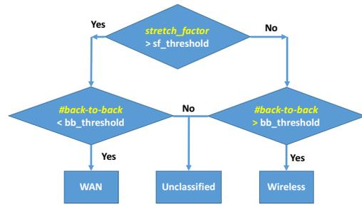
Figure 3: QProbe Algorithm
