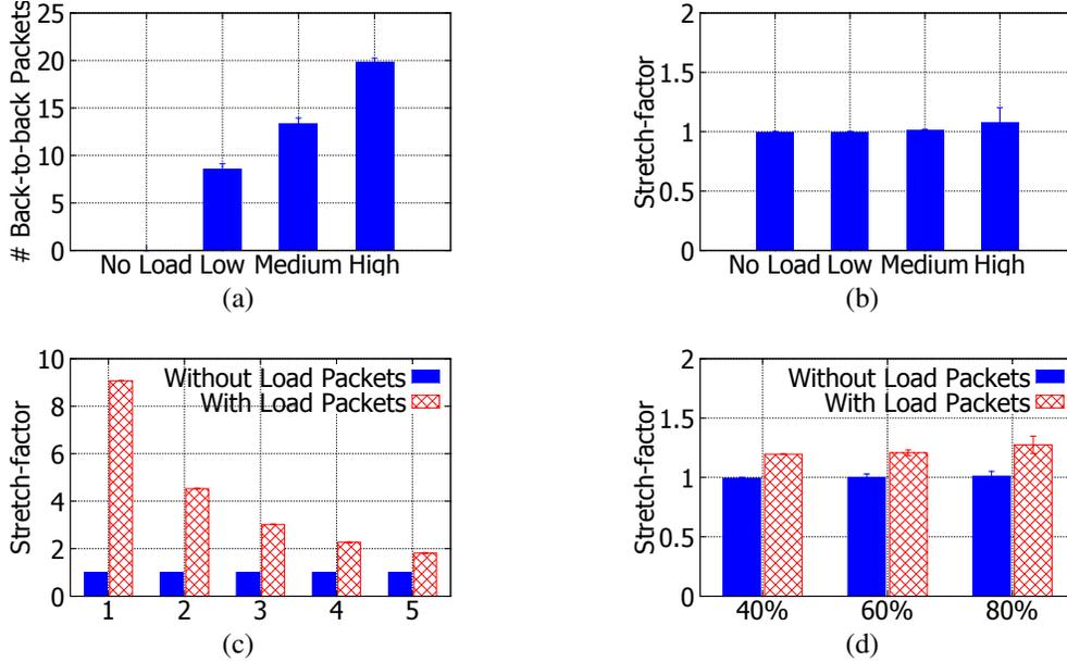
Figure 4: (a) Number of back-to-backs, and (b) *stretch-factor* with varying wireless congestion levels. *stretch-factor* for WAN link bottlenecks due to (c) varying link bandwidth (in Mbps) and (d) varying cross-traffic volumes.
