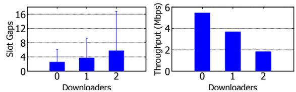
Figure 1: (a) Slot gaps between assignments, and (b) Throughputs observed by the measurement device with different number of background downloaders
