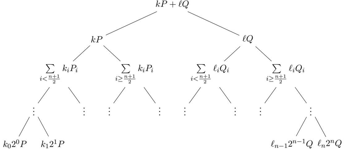
Figure 5: computing  $kP + lQ$ : parallelized double-and-add
