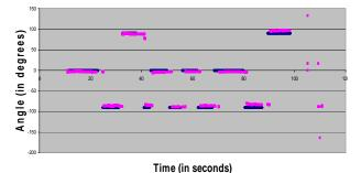
**Figure 4** – sample results on a multi-speaker test. The sources are at 0°, -90°, and +90°.
