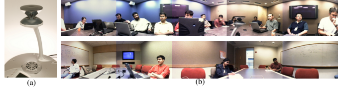
Fig. 1. RoundTable device and its captured images. (a) The RoundTable device. (b) The captured panoramic images.
