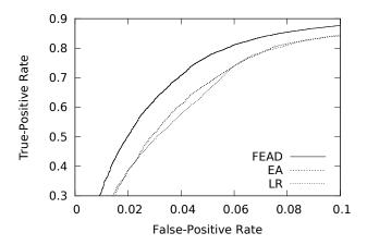
Figure 2: The ROC curves of the baseline (LR), easy adapt (EA) and our ensemble approach (FEAD) when the false-positive rate (FPR) is less than 0.1. The normalized AUC scores of LR, EA and FEAD in this region are 0.592, 0.602 and 0.677, respectively.
