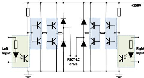
Figure 9: The PSCT-LC H-bridge driver circuit.
