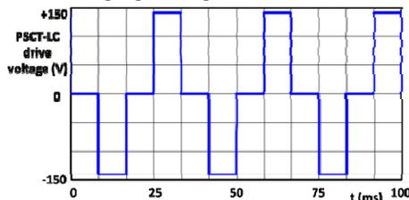
Figure 8: The waveform that drives the PSCT-LC screen. A 150V potential is applied for 8.3ms at a rate of 60Hz; to prevent any DC offset the polarity of this is reversed on alternate cycles.
