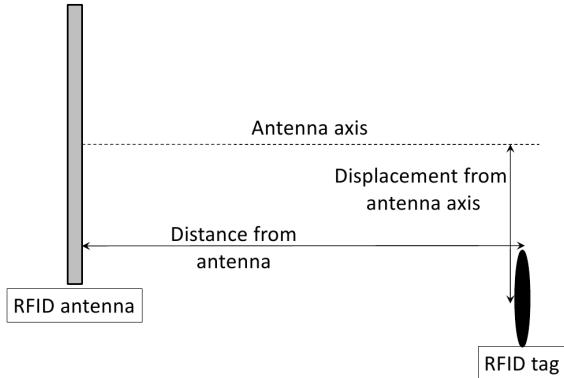
**Figure 3: Measurement setup**
