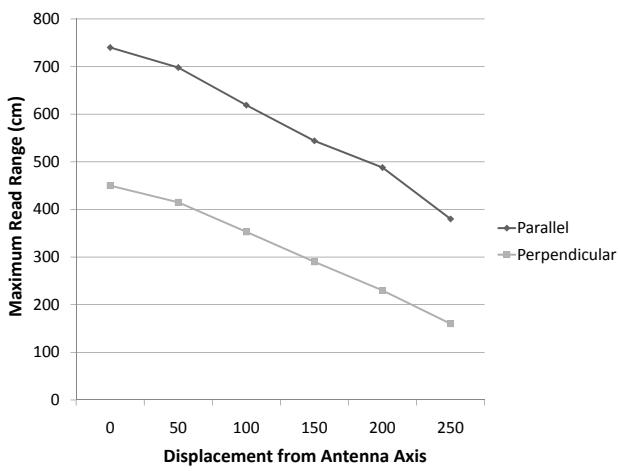
**Figure 4: Effect of displacement from antenna axis on read range**
