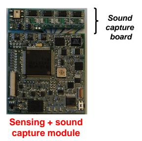
Figure 3. A Prototype LittleRock Board with Sound Capturing Extension. The board has an accelerometer, a digital compass, a gyro, a temperature sensor, and a pressure sensor.
