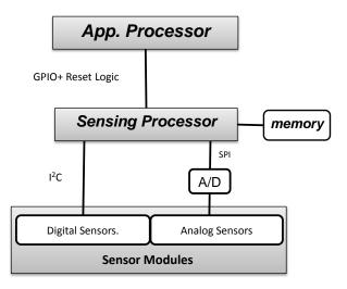
Figure 2. The LittleRock Architecture for Mobile Phones to Enable Continuous Low Power Sensing.
