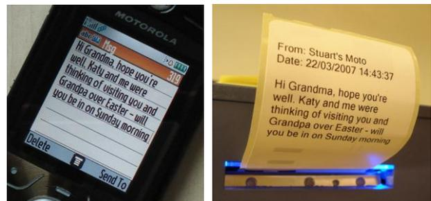
Figure 4. (a) Message being sent from a mobile phone, (b) Txt-it Notes prints the received message
