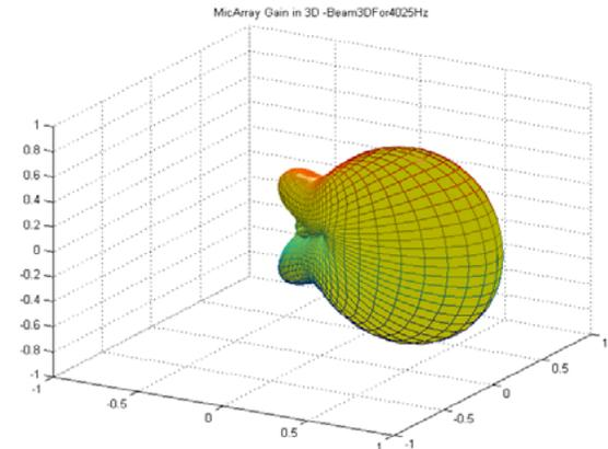
The beam shape in 3D proves frequency independent beamforming
