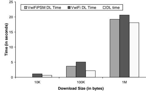
**Figure 3:** Impact of the communication protocol on web page download time at the connected client. The VwifIPSM bar is missing in the 10 KB case because the download finished too quickly for us to be able to reliably interpose VirtualWiFi switching during the download.
