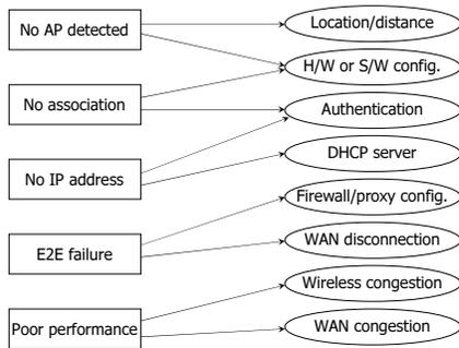
**Figure 1: Problem symptoms observed at a client and some of the associated causes.**
