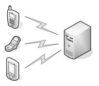
of the speech signal (e.g., Mel-cepstrum), an alternative approach is to put the speech front end on the mobile device and transmit only speech features to the server (Deng et al. 2002), as shown in Figure 4. Transmitting speech features can further save bandwidth because the size of the features is typically much less than that of the compressed audio signals.
