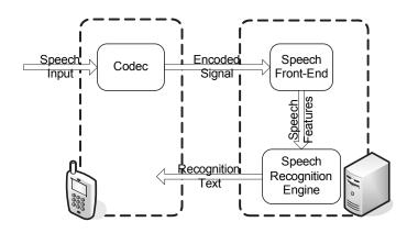
*Figure 3. Distributed speech recognition architecture: speech input is encoded and sent to the server. Speech feature extraction happens at the server side*
