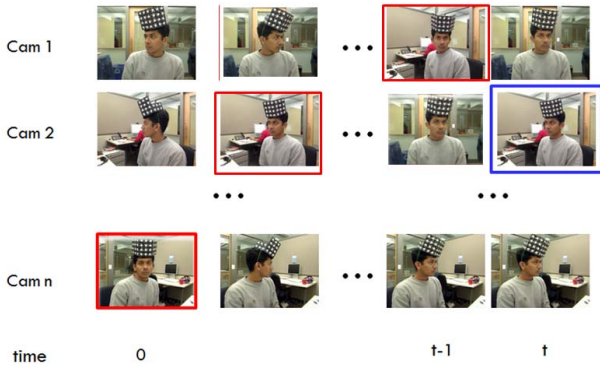
Figure 2. Robustness of a tracking algorithm using reference frames (highlighted in red between t - 1, \dots, 0 , the current frame is highlighted in blue rectangle) temporally and spatially across cameras.
