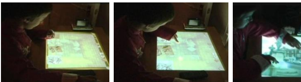
Figure 7: Interacting with digital objects. Switching from interacting with a mouse (left), to hybrid bimanual interaction using touch and mouse (middle), to bimanual touch input.
