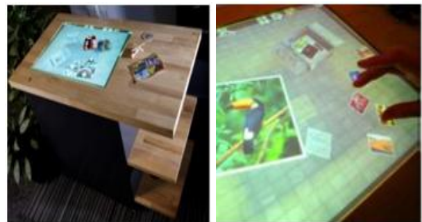
Figure 1: Our interactive surface, a bespoke tabletop, with an embedded multi-touch display and overhead camera for imaging physical objects on the surface (left), with a custom physics-enabled photo application (right).
